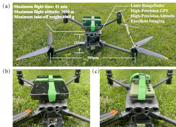
Fig. 2. UAV and measurement devices: (a) UAV equipped with measurement devices; (b) Base station switchable device; and (c) Base station fixed device.
